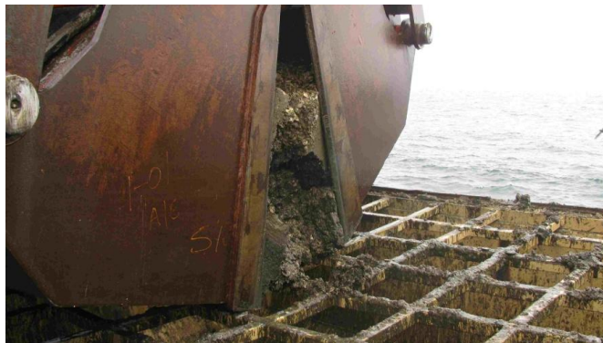
Grab unloading into the hopper
