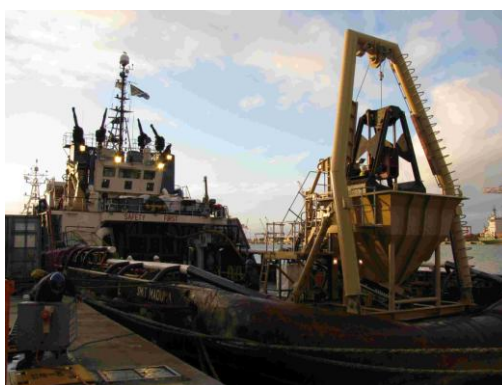
MV Smit Madura with grab installed
