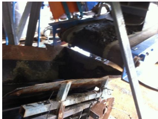
Figure 2: ROM feed into the screening process
