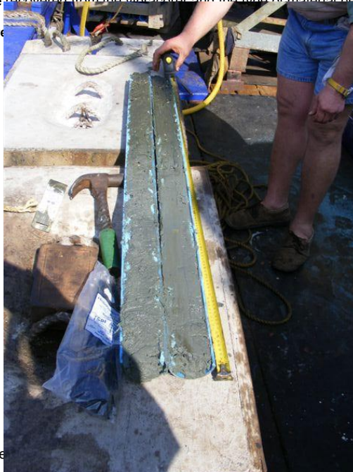
Figure 2.5 Core recovered from the vibrocorer and the type of material being sampled.
