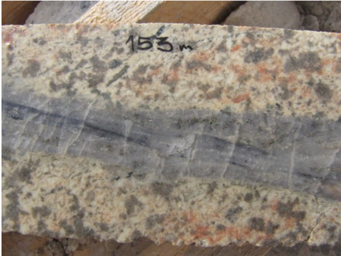
Figure 4. Typical Stockwork Quartz Vein with Pyrite, Chalcopyrite and Molybdenum Selvedge
