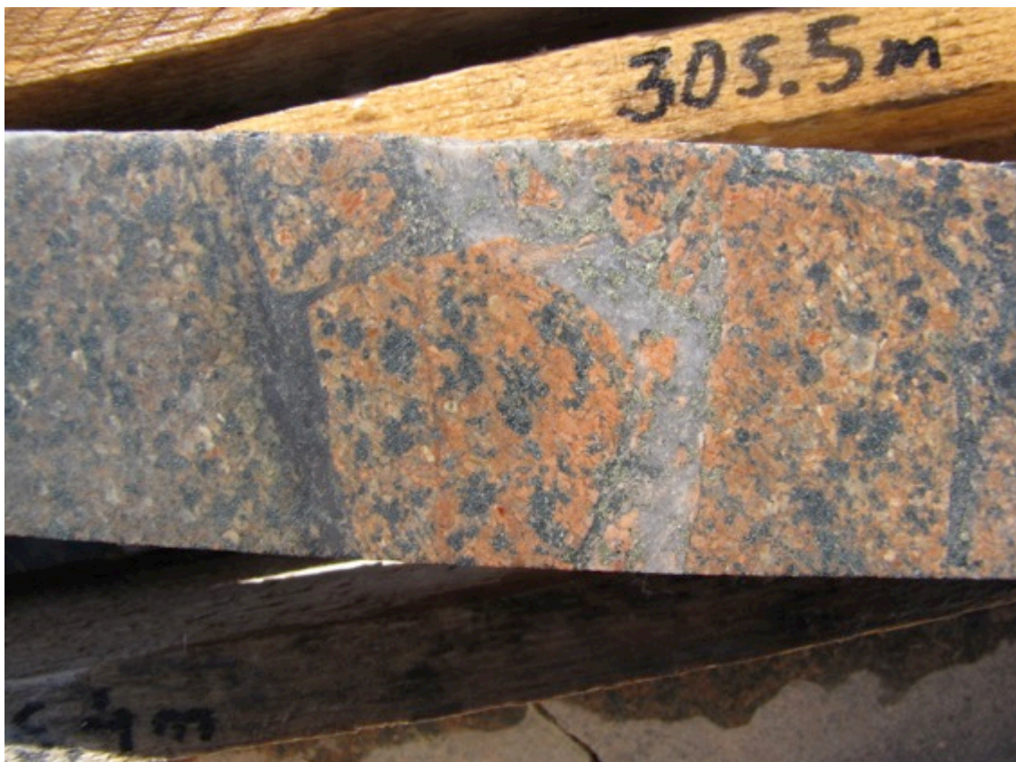
Figure 3. Mineralised Quartz Vein in Potassic Alteration with Hydrothermal Magnetite
