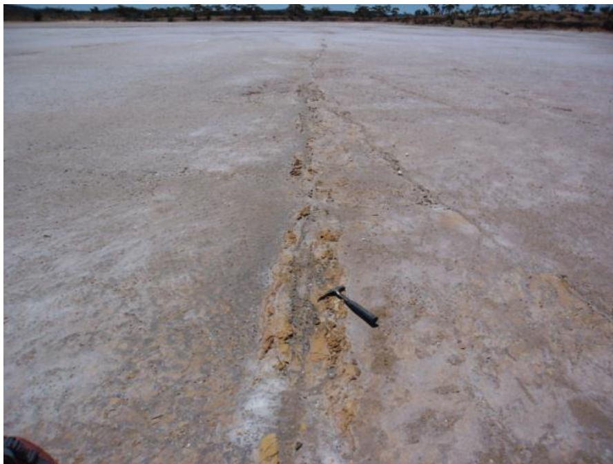
Figure 4 A 30 cm wide vertical quartz vein assayed 24.1 g/t with visible gold present
