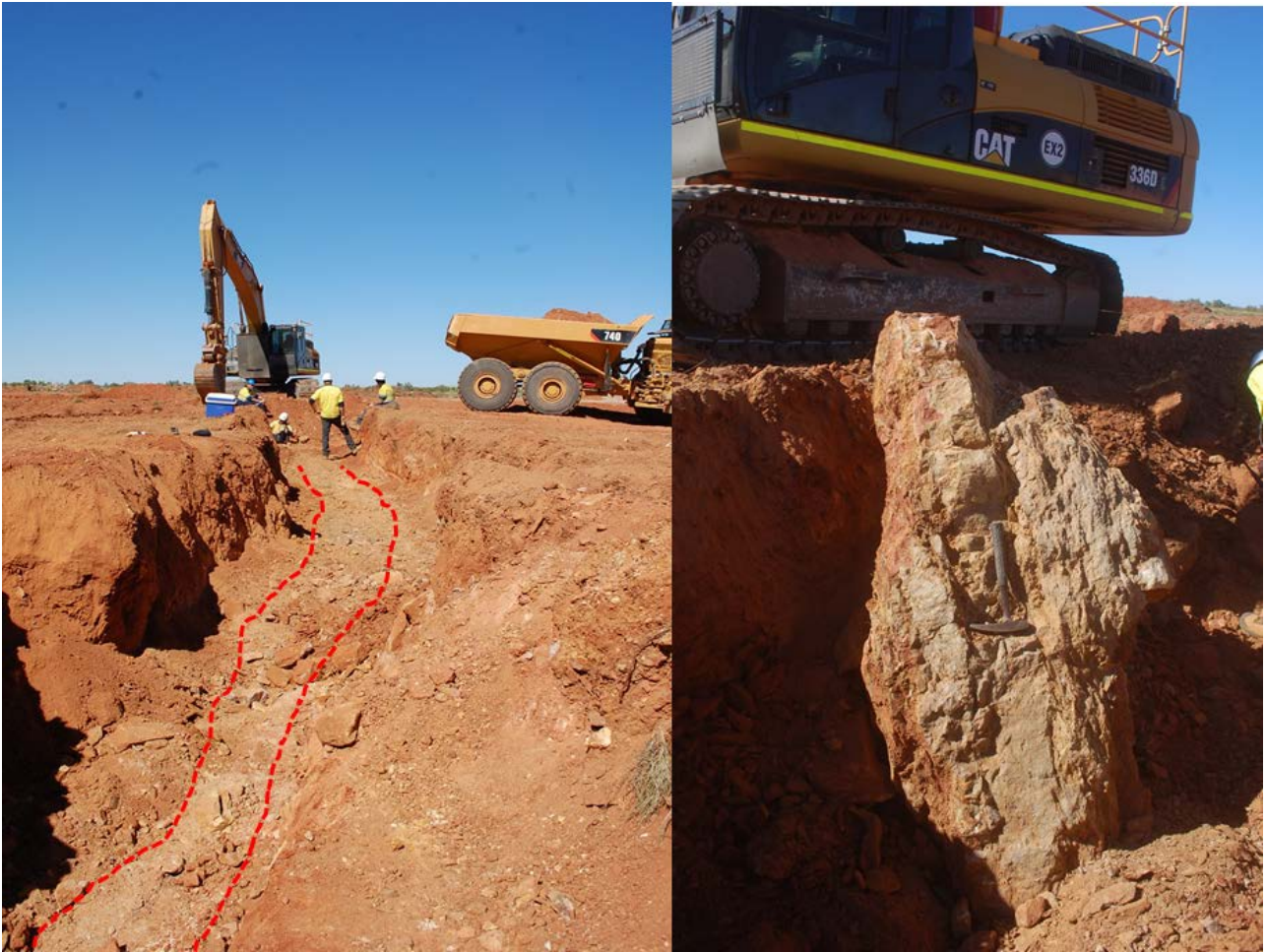
Figure 5. Excavation of high-grade veins from Golden Hind. Left image shows the first bench at the Golden Hind with vein extracted via trench and revealed in the floor of the trench. Right image shows a ~3 tonne piece of high-grade vein from Golden Hind containing abundant visible gold; entire block is quartz with multiple vein phases.
