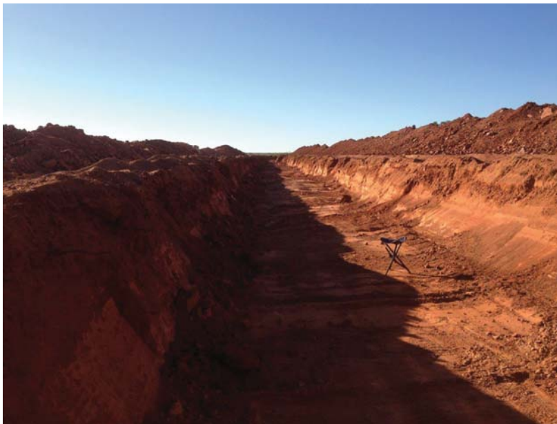
Figure 8. Gold-bearing vein material and waste extracted from 240 metres of strike length (first bench) at the Western Limb. Material on the left surface is stock-piled high-grade vein, and on the right is waste material or material being resampled to check for presence of gold.
