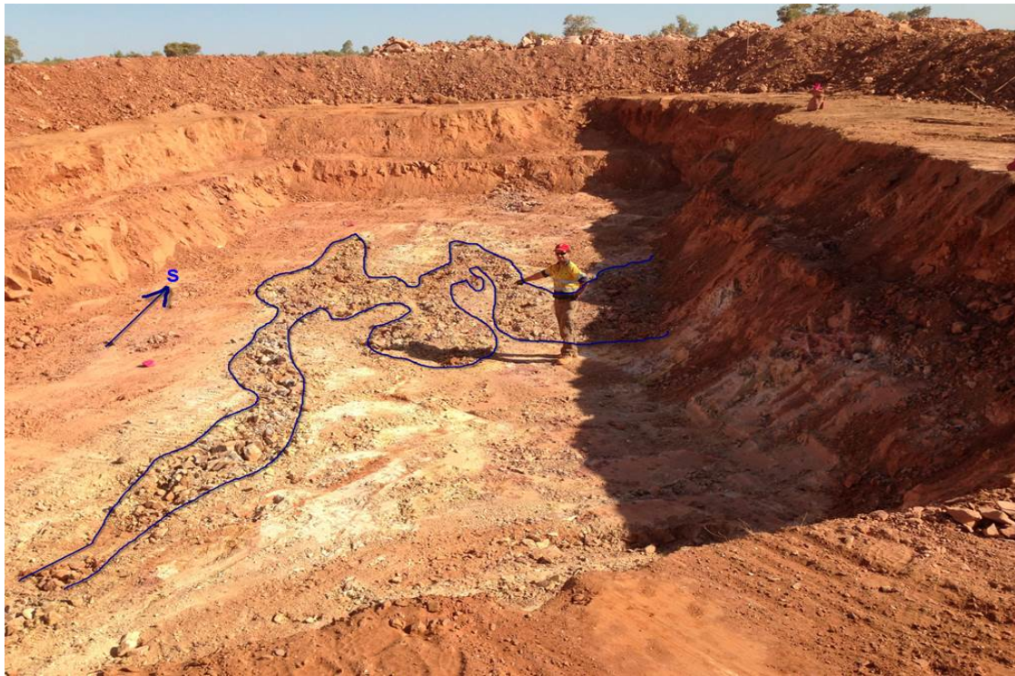
Figure 3. Old Pirate South area showing southerly plunging fold nose (blue outline is quartz vein).
