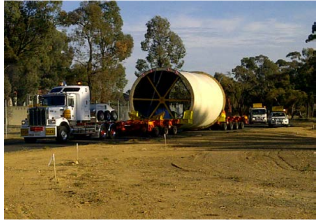
Ball mill shell arriving at site
