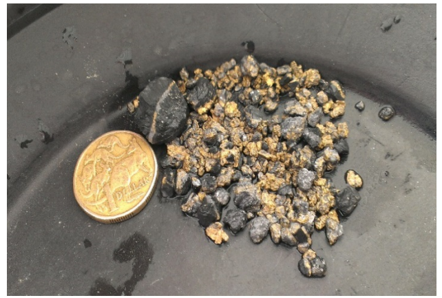
Coarse free gold in RC hole PE873 (194-195m)
