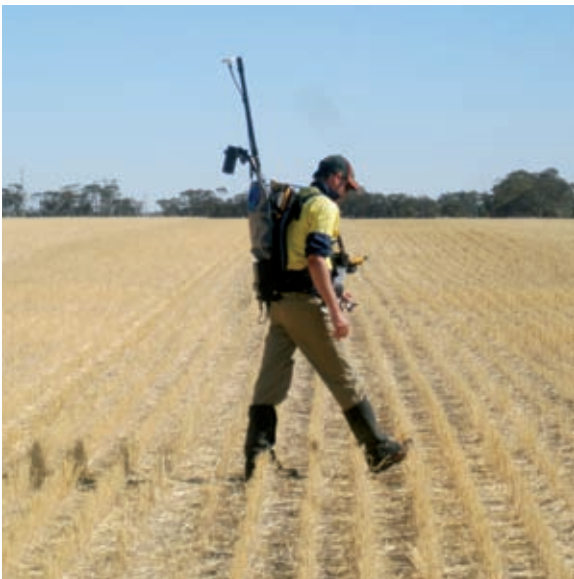
Ground magnetic survey operations following crop harvesting
