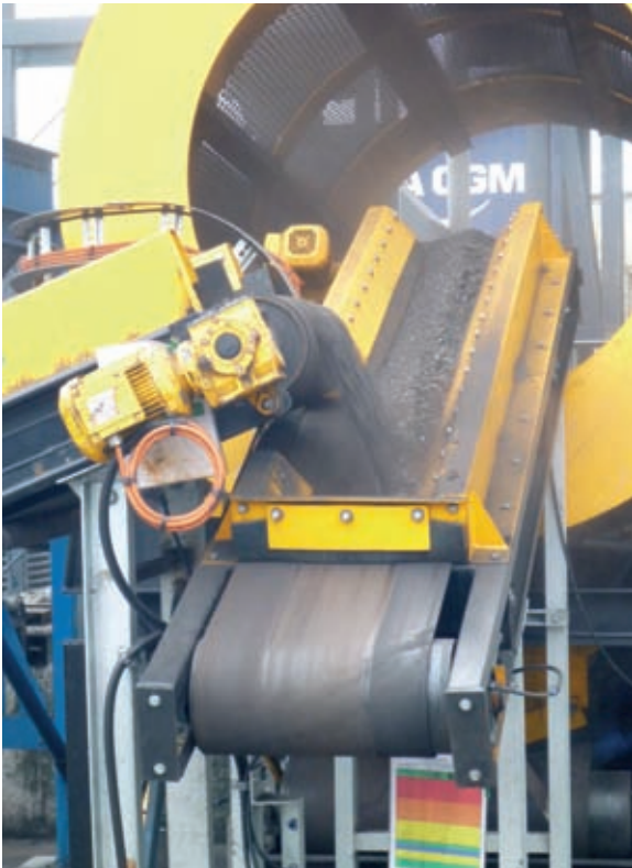
Feeding mill scale into the trommel
