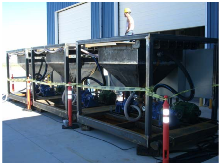
Figure 1 – Initial hydraulic flow tests being undertaken on the 3 interconnected Ablation modules that will comprise part of the 5tph Ablation Unit that is nearing completion.
