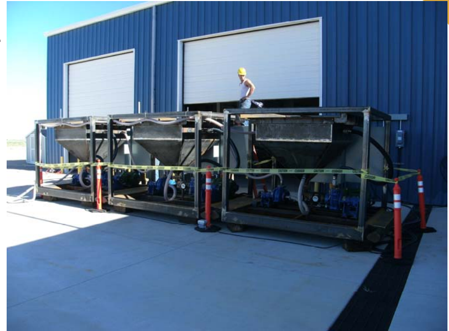
Initial tests being undertaken on the 3 interconnected Ablation modules constructed for the 5tph Unit.
