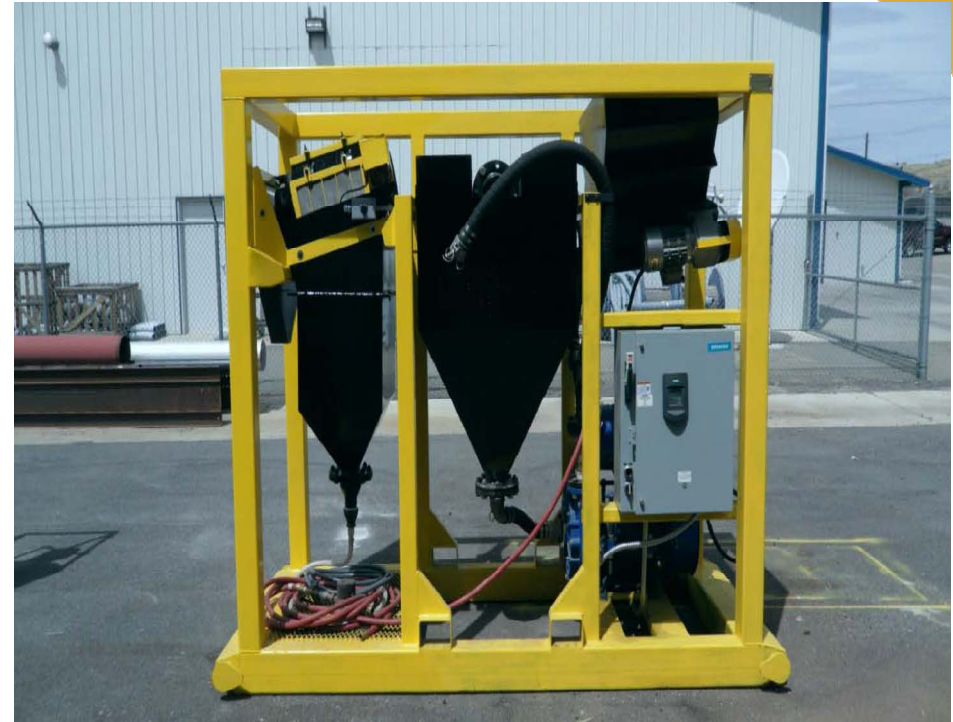
Pilot-scale Ablation unit that processes ~0.5 tonnes/hour. This technology is being scaled up to units that can process ~5 tonnes/hour.
