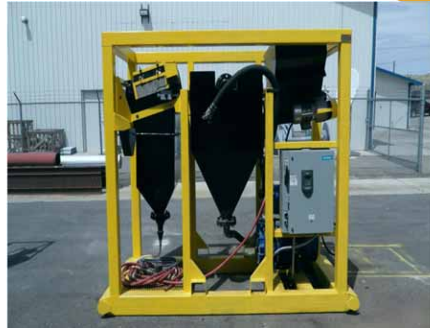
Pilot-scale Ablation unit that processes ~0.5 tonnes/hour. This technology is being scaled up to units that can process ~5 tonnes/hour.
