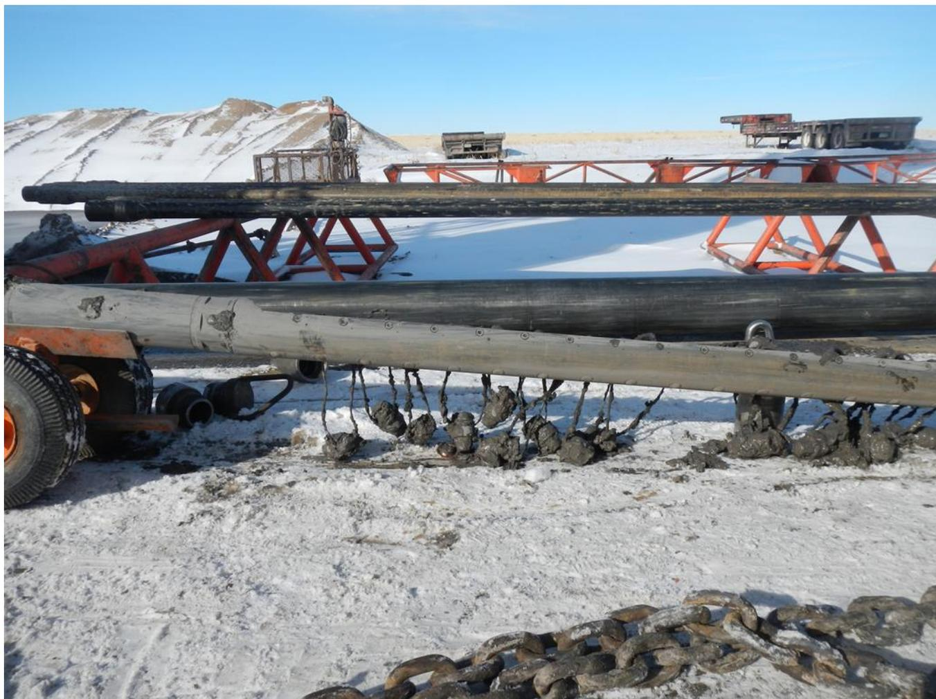
Side Wall Core Gun from QCWR 34-3 (Niobrara and Codell test work)
