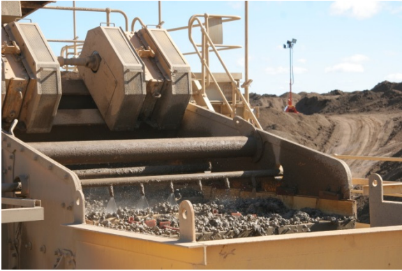
Screen oversize ore – log washer discharge
