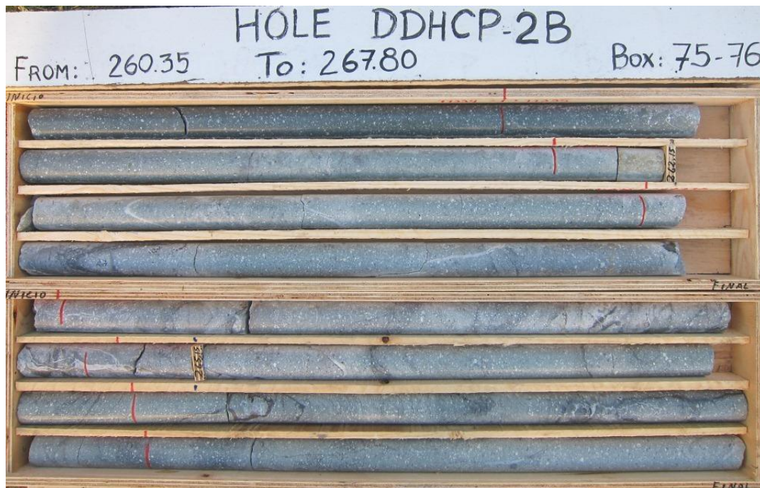
Figure 5: Porphyritic dacite with pyrite-filled fractures, grey-black veinlets of silver sulphosalts and chalcopyrite.
