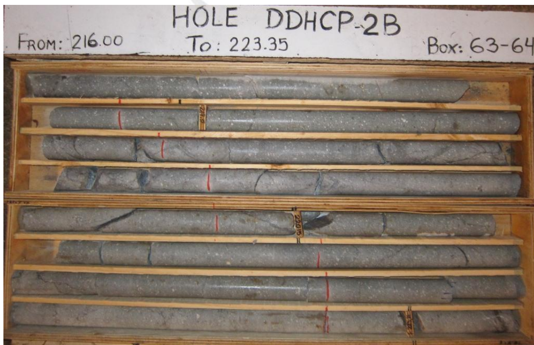
Figure 4: Porphyritic dacite with fine calcite and fine pyrite veining and disseminated pyrite 216-223.35m
