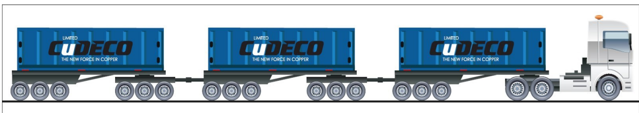
Figure 2: Schematic diagram of typical Type 2 road-train configuration, with specially designed fully sealed containers.
