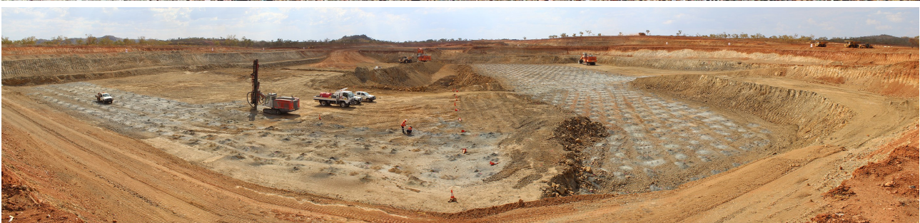
Figure 1: Significant quantities of coarse native copper (99.8% Cu) and the high-grade copper mineral cuprite (88.8% Cu) is being encountered in blast-hole drilling within resource drilling voids (see Figure 4). Bottom image shows Stage-1 of the LM Starter Pit underway, with blast-hole drilling predominately in waste (left and right) and in ore (darker drilling spoils centre).
