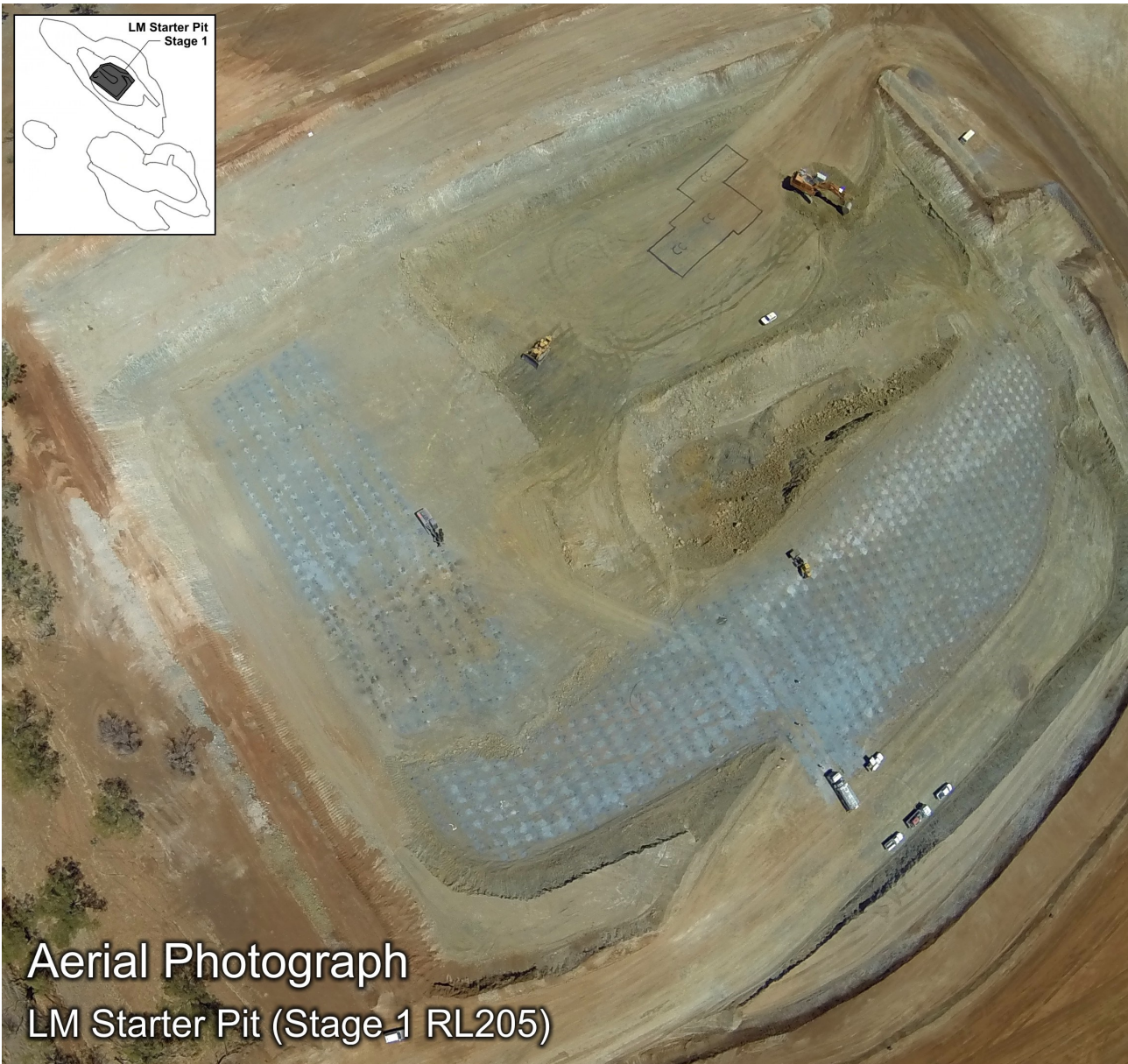
Figure 6: Aerial view over LM Starter Pit (Stage 1) - blast-hole drilling and previously excavated box-cut which finished approximately 10m below the current pit floor.
