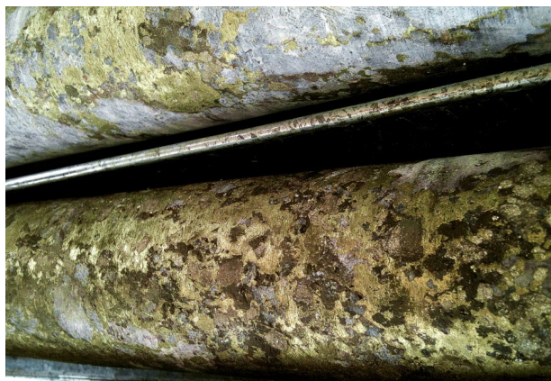
Figure 4: Diamond Drill core DODH457 (currently drilling); example of high-grade copper mineralisation (massive to semi-massive chalcopyrite) from approximately 185-186m - chalcopyrite (34.6% copper metal) chalcocite (79.9% copper metal)
