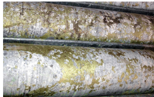
Figure 3: Diamond Drill core DODH456 showing semi-massive chalcopyrite in calcite/quartz breccia from approximately 160-162m that returned assay results of 7.66% Cu - chalcopyrite (34.6% copper metal)
