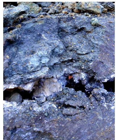
Figure 7: High-grade chalcocite suitable for Direct Shipping Ore (DSO) being excavated from the base of the Las Minerale Starter Pit, with estimated grades ranging from 20-60% copper, based on visual estimates, confirmed with XRF analysis. Image of XRF showing 54.7% Cu result from the face of a large chalcocite boulder.
