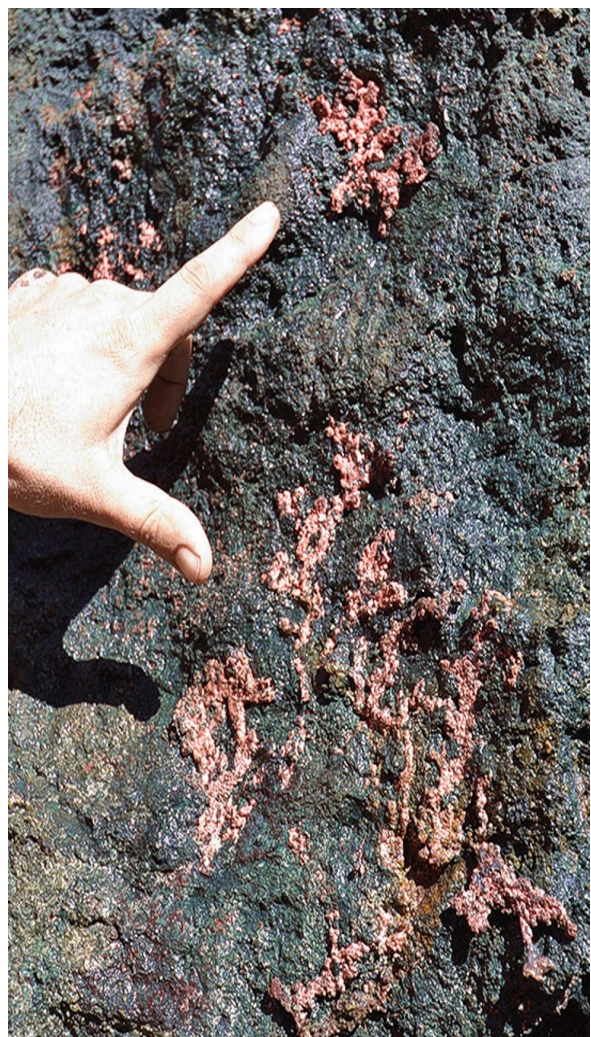
Figure 4: Above; native copper masses associated with chalcocite exposed in the face of the Las Minerale Starter Pit and below; close-up detail of native copper.
