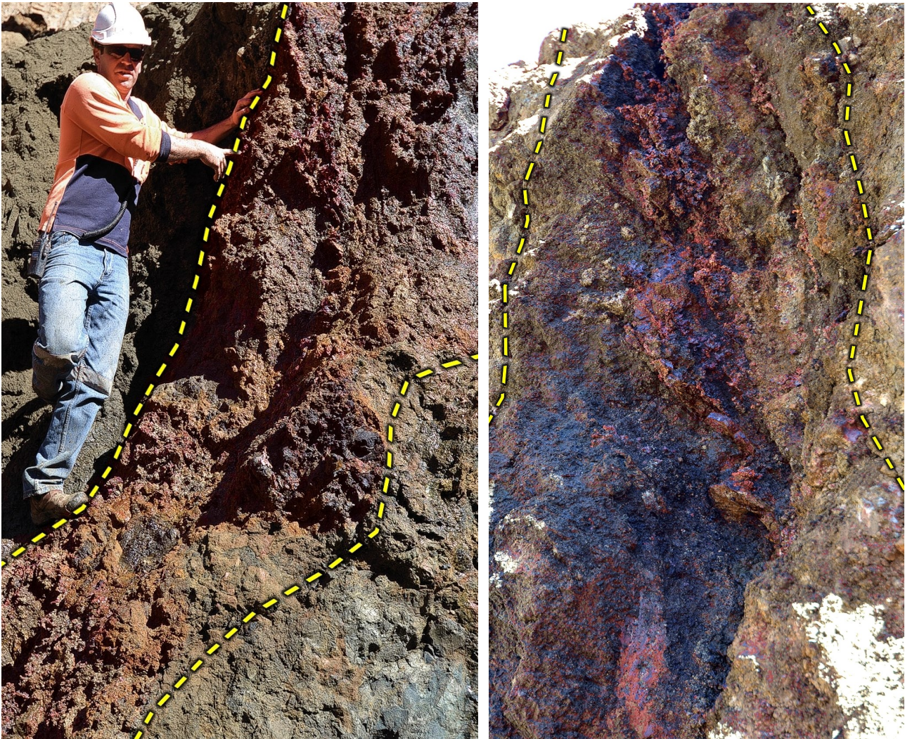
Figure 1: Examples of separate large coarse native copper agglomerates currently being unearthed at the Las Minerale Starter Pit, just 15-20m below surface. Image to the left shows zone of high-grade native copper and cuprite that has been mapped at the base of the pit for over 25m. The image to the right shows soft sooty chalcocite crystals (blue-grey colour) falling out of voids within the coarse native copper like confetti down the face of the excavation...it is thought that during exploration drilling, much of this soft sooty chalcocite washed out of the vuggy drill-core due to high pressures required to maintain water returns during drilling, and has not been included in assay results. Native copper contains 99.65% Cu, cuprite contains 88.8% Cu and chalcocite contains 79.85% Cu.
