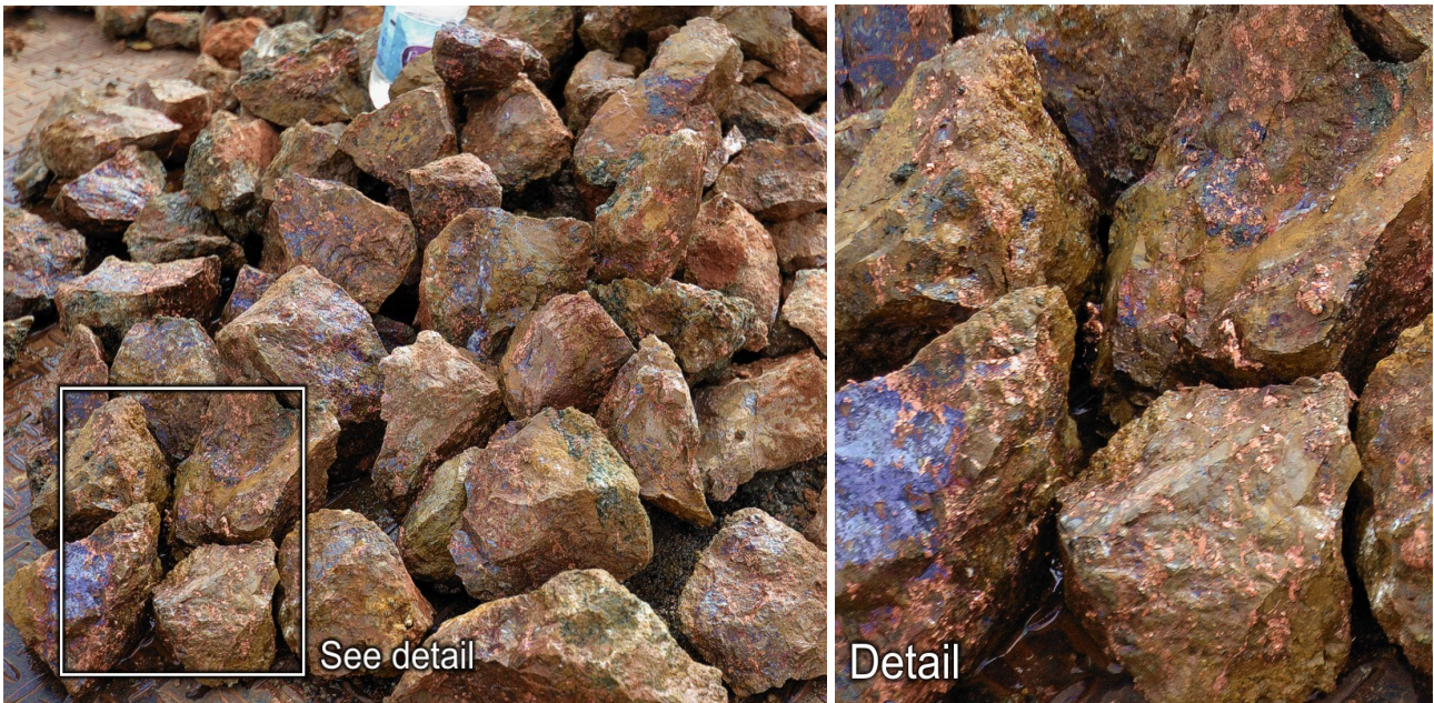
Figure 10: Example of DSO suitable crushed native copper ore (wet) - sample from large 3 tonne agglomerated mass of native copper, after being processed through the coarse screen (<120mm) stage of the Company's mobile crushing circuit. The sample is estimated to contain 40% Cu from a combination of copper species including native copper (99.65% Cu), cuprite (88.8% Cu), and chalcocite (79.85% Cu) +/- malachite, azurite and minor chalcopyrite.
