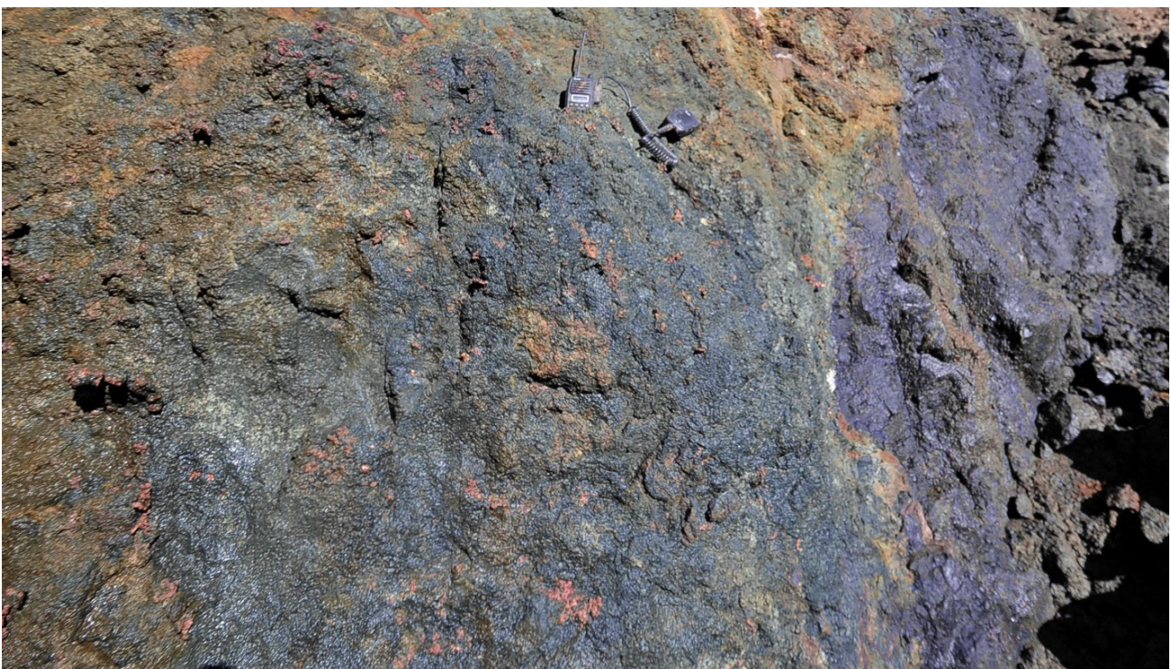
Figure 24: High-grade ore face at the base of the Las Minerale Pit - Coarse native copper in grey-green clays (left and middle) and high-grade chalcocite ore (right in background). Field of view approximately 8m from left to right.
