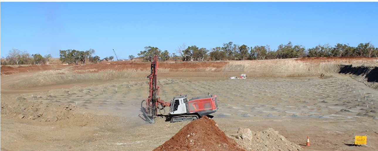
Figure 19: Blast-hole drilling has commenced in waste areas adjacent to the main ore zones at Las Minerale - ore areas are still free-dig at this stage.
