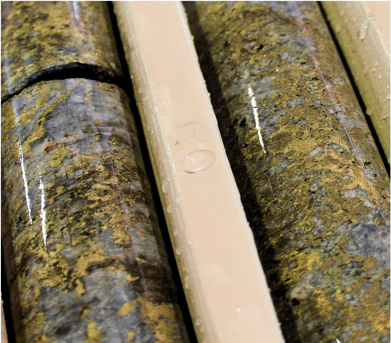
Figure 2: Diamond drill core DODH474 (dry core) showing semi-massive and disseminated sulphides (chalcopyrite and pyrite) in calcite/quartz/siltstone breccia from approximately 210-211m - chalcopyrite contains 34.6% copper metal and pyrite is typically associated with cobalt at Rocklands.
