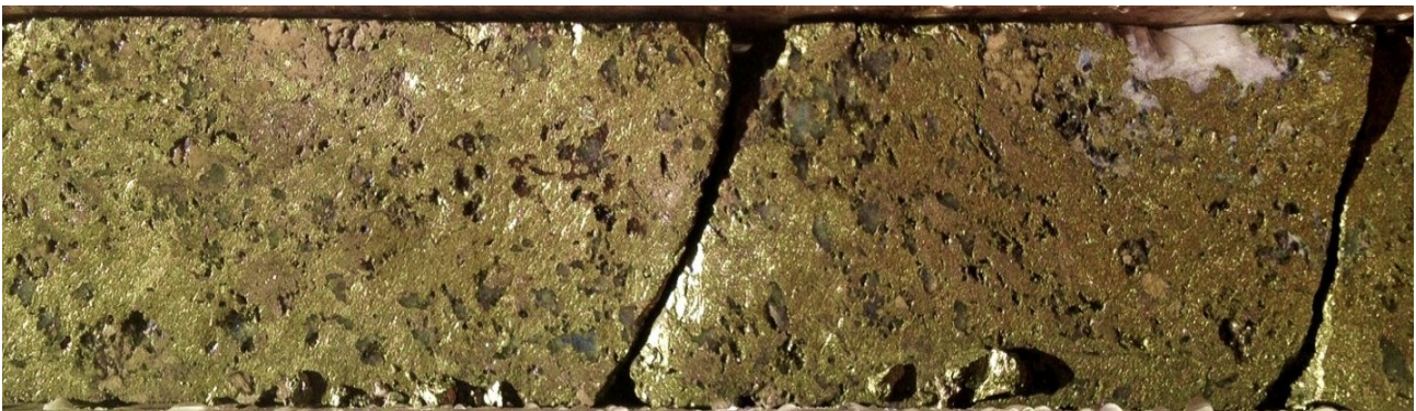
Figure 1: Diamond drill core DODH472 (wet core) showing massive chalcocpyrite and pyrite in calcite/quartz breccia at approximately 187-188m which assayed 9.98% Cu.
