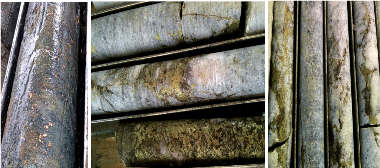
Figure 4: Diamond Drill core DODH457, left to right; native copper and chalcocite at approximately 33m and massive to semi-massive chalcopyrite from approximately 186-188m and 179-182m - chalcopyrite (34.6% copper metal) chalcocite (79.9% copper metal).
