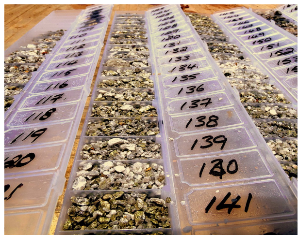
Figure 5: Metre after metre of high grade copper mineralisation intersected in wide-diameter pit-dewatering drill hole NVB038 - chalcopyrite (34.6% Cu metal) chalcocite (79.9% Cu metal) bornite (63.3% Cu metal) in hydrothermal breccia (assays awaited).
