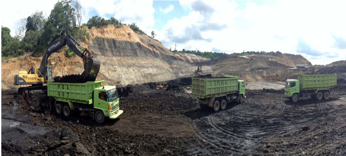
Figure 1: Photograph showing coal being extracted from Seam B in the foreground whilst Seam A is shown exposed at a higher elevation (background).
