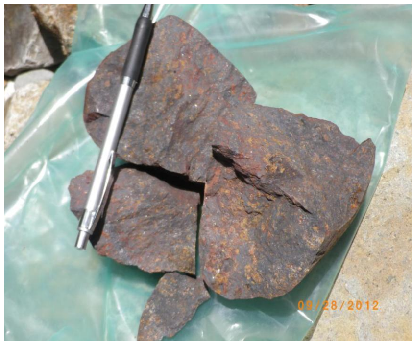
Photo3: Wara Ck iron ore prospect sample with magnetite and > 50% Fe
