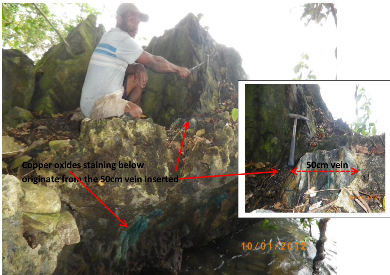
Photo 1: Outcrop at the Pulding Cu/Mo IOCG prospect with petrography of samples describing quartz/tourmaline/albite alteration with primary chalcopyrite
