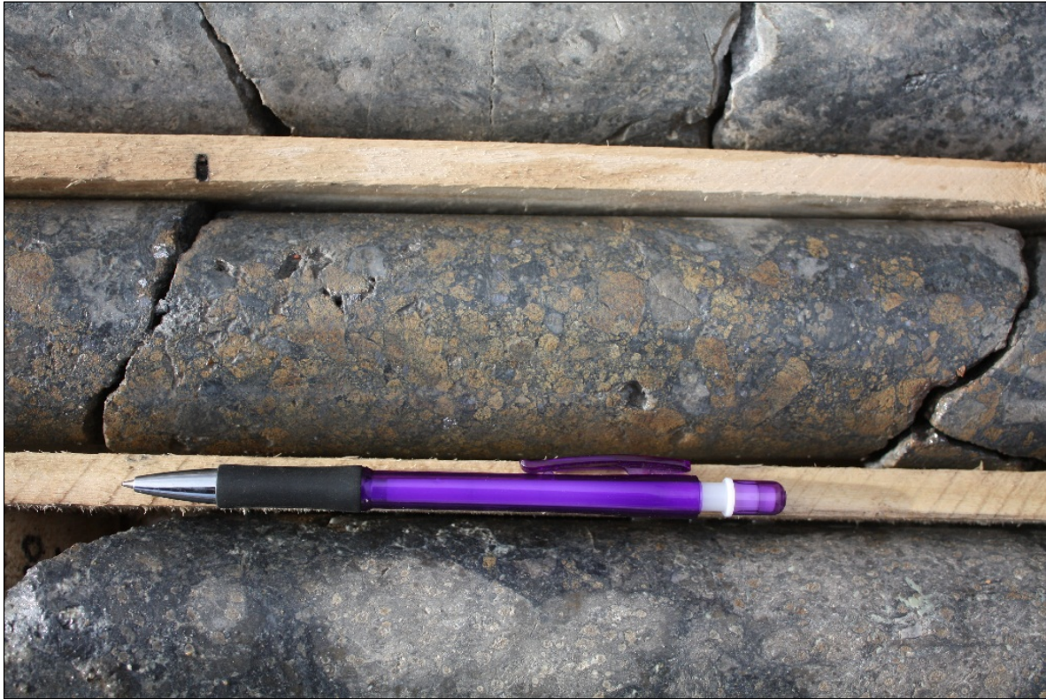
Figure 1: SM 13-16. Breccia at 135.8m with matrix of predominantly galena and yellow sphalerite with minor pyrite and arsenopyrite
