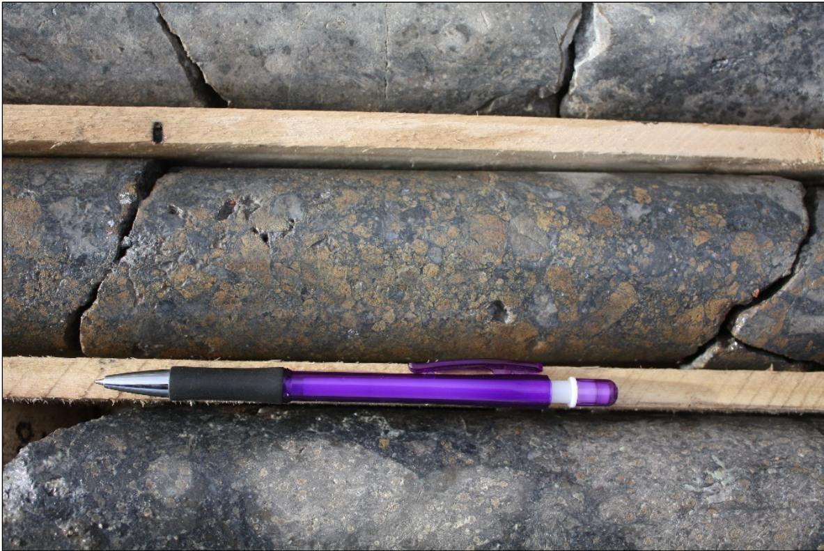
Figure 9: SM 13-16. Breccia at 135.8m with matrix of predominantly galena and yellow sphalerite with minor pyrite and arsenopyrite
