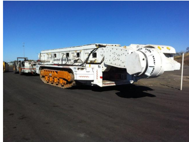
Largest capacity and most flexible shield transport configuration – 57t 2m wide with power assist hydraulic trailer wheel
