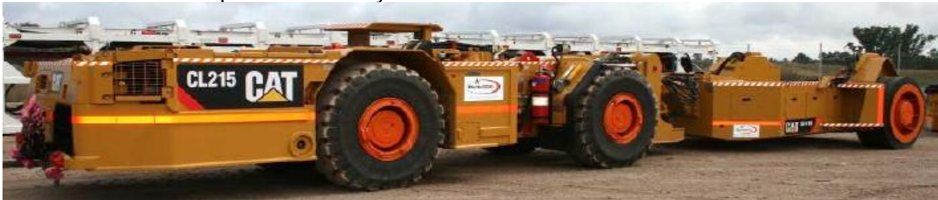
Largest capacity and most flexible shield transport configuration – 57t 2m wide with power assist hydraulic trailer wheel
