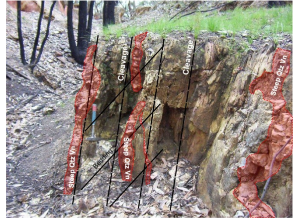
Steep cleavage parallel quartz vein set within historic open cut workings (Grey Horse Line).
