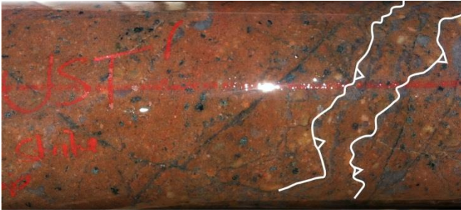
DUNDD012 - 990m DEPTH (UST - Down Hole) (North - South Strike and approx 20° W Dip)
