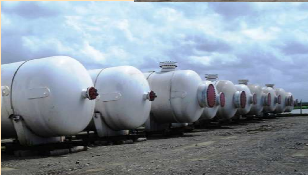
Mixed Refrigerant System Drums
