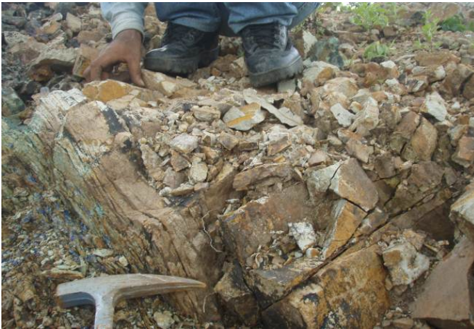
Figure 9: Sample site B120, contact aplitic dyke and sample B119 which assayed 4.78% Cu, 0.14% Zn and 0.7ppm Ag per tonne over the 0.5 metre interval sampled. The dyke was sampled over 0.5 metres to assess disseminated mineralisation in the 'footwall'. The dyke contained 2.6 times more Cu than what was regarded as the main mineralised zone.
