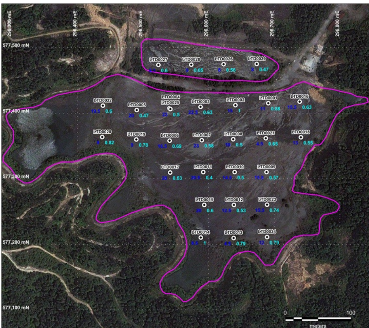
Figure: Tailings drilling collar plan showing outline of the two dams used in the resource model (pink). Completed collars shown as black symbols with Depth to Basement annotated in dark blue and average gold grade for each hole in light blue. The average gold grade excludes assays from basement material.
