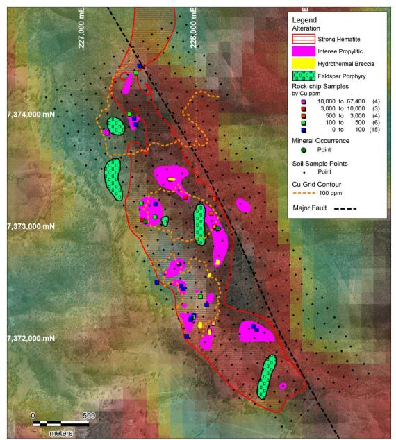
Figure 2: Alteration distribution at Oakey Creek prospect. Broad and continuous zone of hematite alteration encloses extensive areas of intense propyllitic-style alteration with localised hydrothermal breccia development. Merged radiometric K:Th image and GeoEye satellite image as background.
