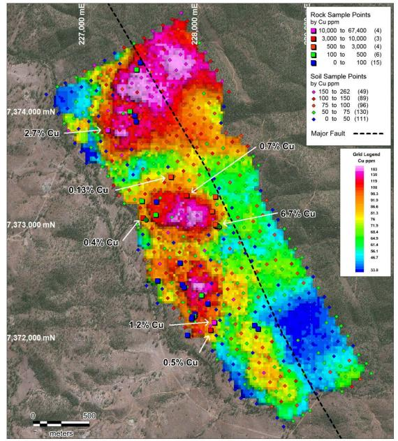
Figure 1: Copper in soil at Oakey Creek prospect. Gridded (Kriged) Cu soil data with rock-chip sample points and Cu assay callouts. GeoEye satellite image as background.
