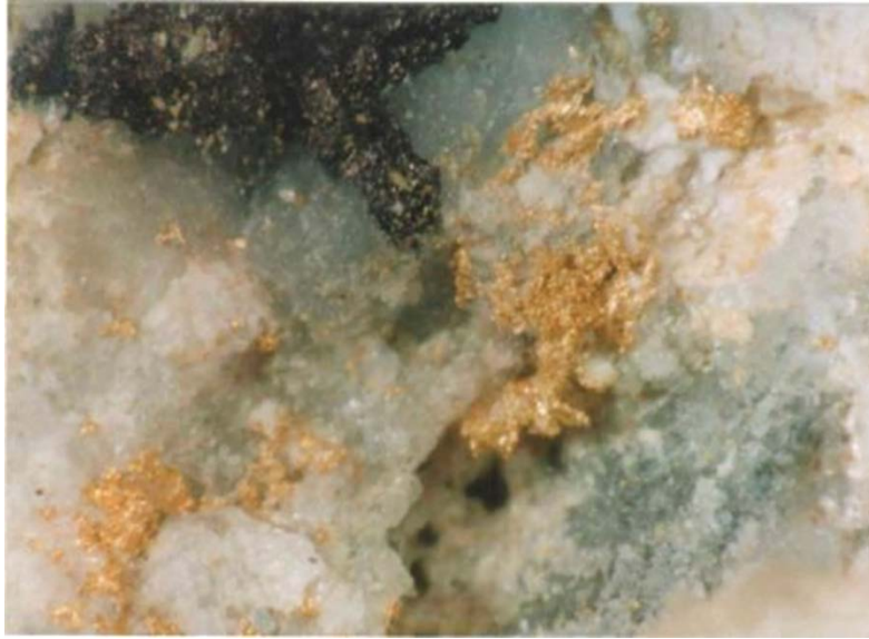
Photograph; Dendritic gold on quartz. Sample M446 (Field of view approx 5mm), Henney et al 1994 pp33, Characterisation of Gold from Lubuk Mandi ,British Geological Survey Technical Report WC94021
