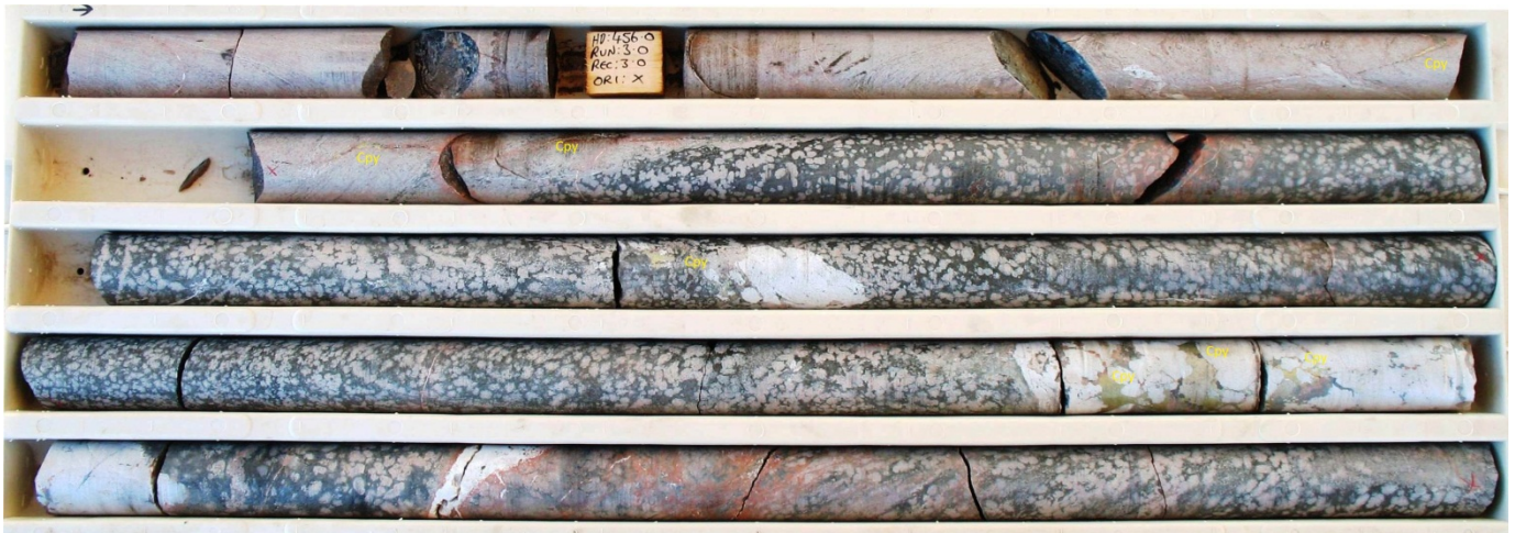
Figure: Drill core from BNG007, 455.5-460m down-hole. Chalcopyrite associated with pyrite-magnetite-quartz in a chlorite-scapolite- altered mafic interval within foliated fine-grained felsic host.
