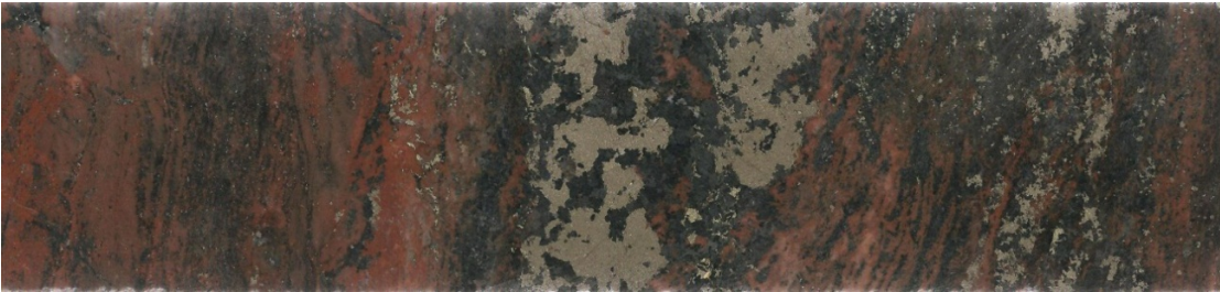
Photographs: Top, chalcopyrite-pyrite mineralisation in quartz-carbonate-feldspar vein. From MMA001 (NQ diamond drill core). Bottom, Ernest Henry style 'Red Rock' alteration with magnetite-pyrite-chalcopyrite-molybdenite. From MMA002 (NQ diamond drill core).
