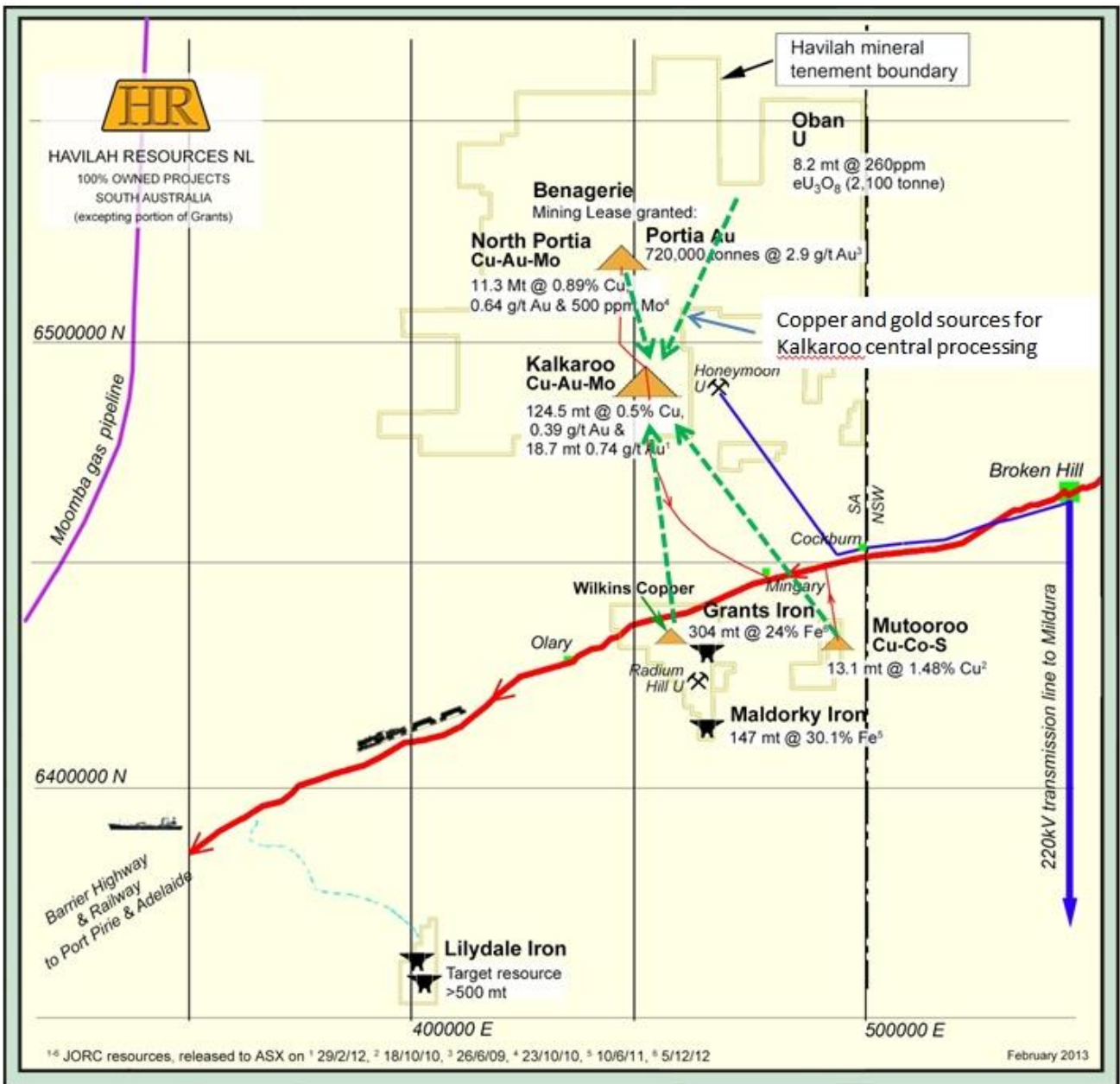
Showing potential sources of copper and gold ore from surrounding projects for a centrally located processing plant at Kalkaroo.
