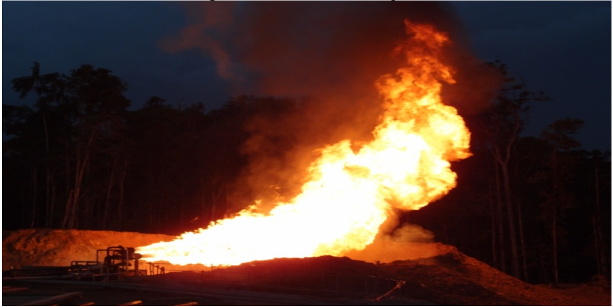
Tingu-1 flow test with Parker Rig 226
