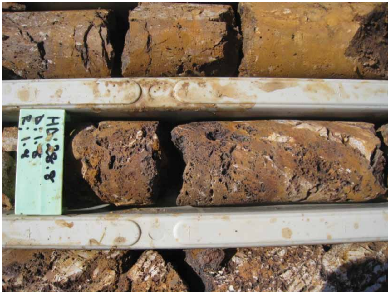
Figure 4 – Typical oxide ore from Golden Camel metallurgical hole MET3 (7.90g/t Au from 28.5 - 29.0m)
