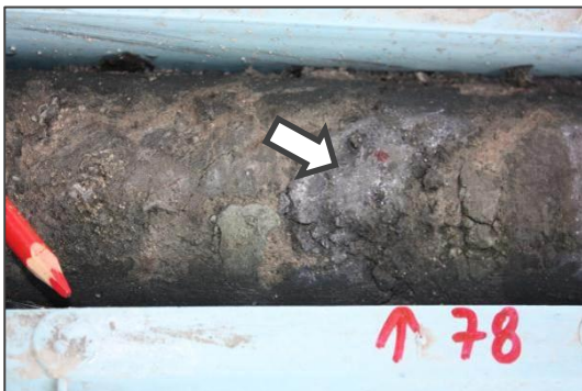
Photo 5: Galena (lead sulphide associated with silver) rich sulphide clast (arrow) (PPDH097 – 78m)
