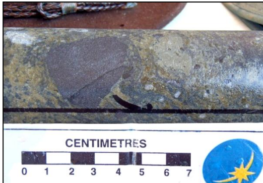
Photo 1: Relatively unaltered flow-banded rhyolite breccia. Pre-alteration basal volcanic - typically anomalous in fluorite, rare earth elements & uranium (PPDH001 – 130m)
