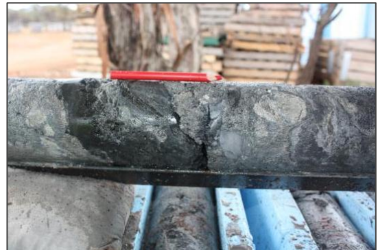
Photo 4: Heterolithic (mixed) breccia with massive sulphide clast (rear of pencil) with quartz & granite clasts (PPDH097)
