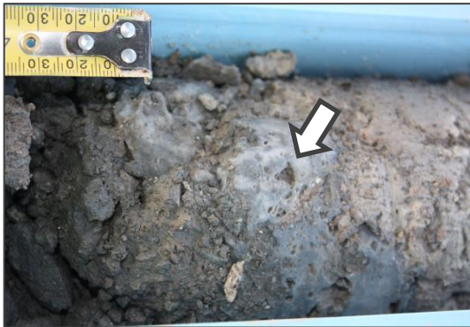
Photo 3: Hydrothermal breccia with dark grey sulphide mineralisation & vuggy silica clasts (arrow) (PPDH091)
