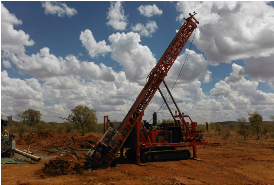
Figure 3 Track mounted diamond rig drilling at Jervois
