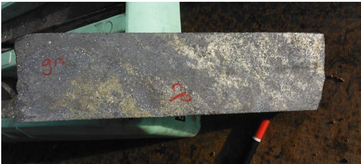
Figure 1 Section of core from hole KJCD048 showing massive copper (cp) and lead (gn) sulphide
