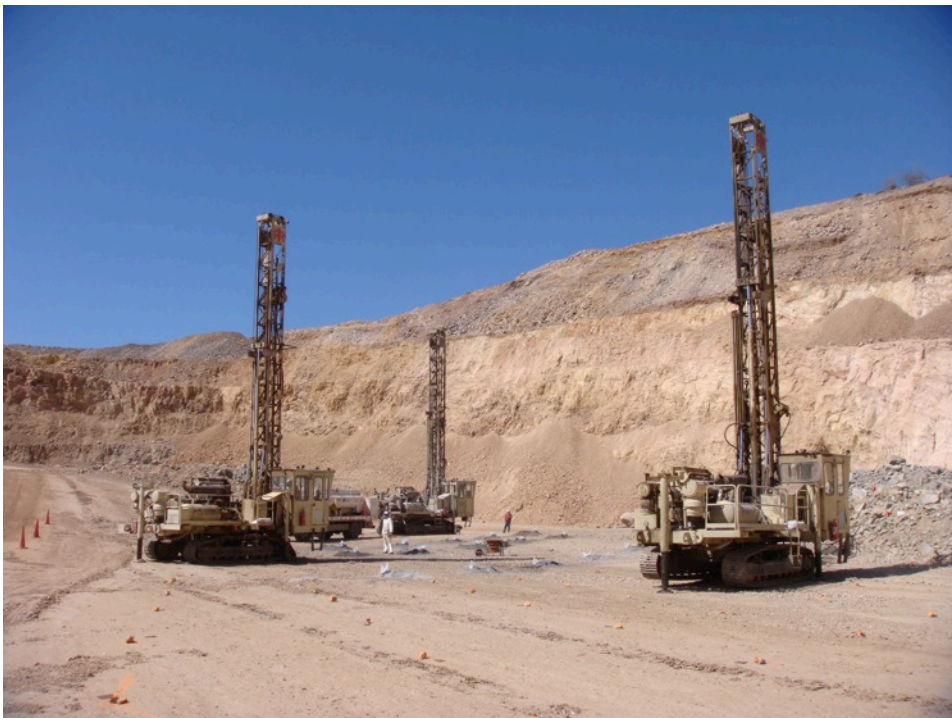
Figure 3 – Owner Mining Drill and Blast Rigs Operating in Tres Perlas Pit
