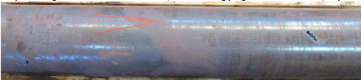
Drill intersection of hematite at Snelgrove Lake - discovery hole MM-13-05
