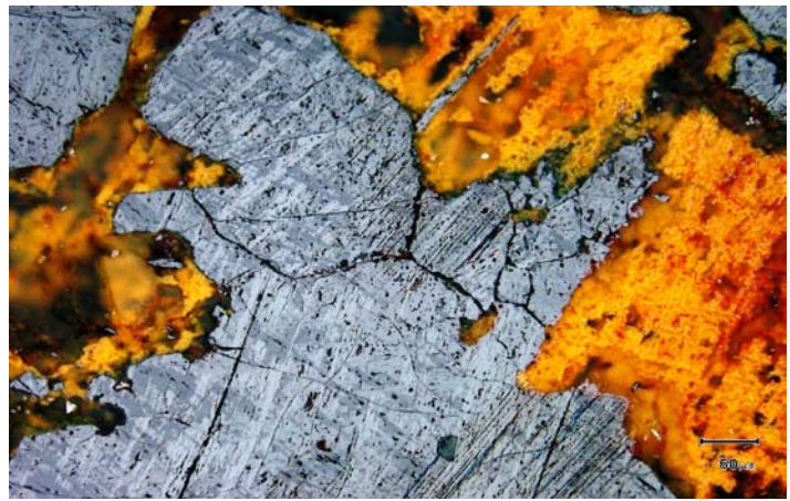
Figure 2: Thin section from hematite sample (left). Bright to mid-grey crystals of hematite with diagnostic cross-hatch fabric. Orange-reddish internal reflections within ex-Fe-silicates, oxidised to earthy goethite-limonite.
