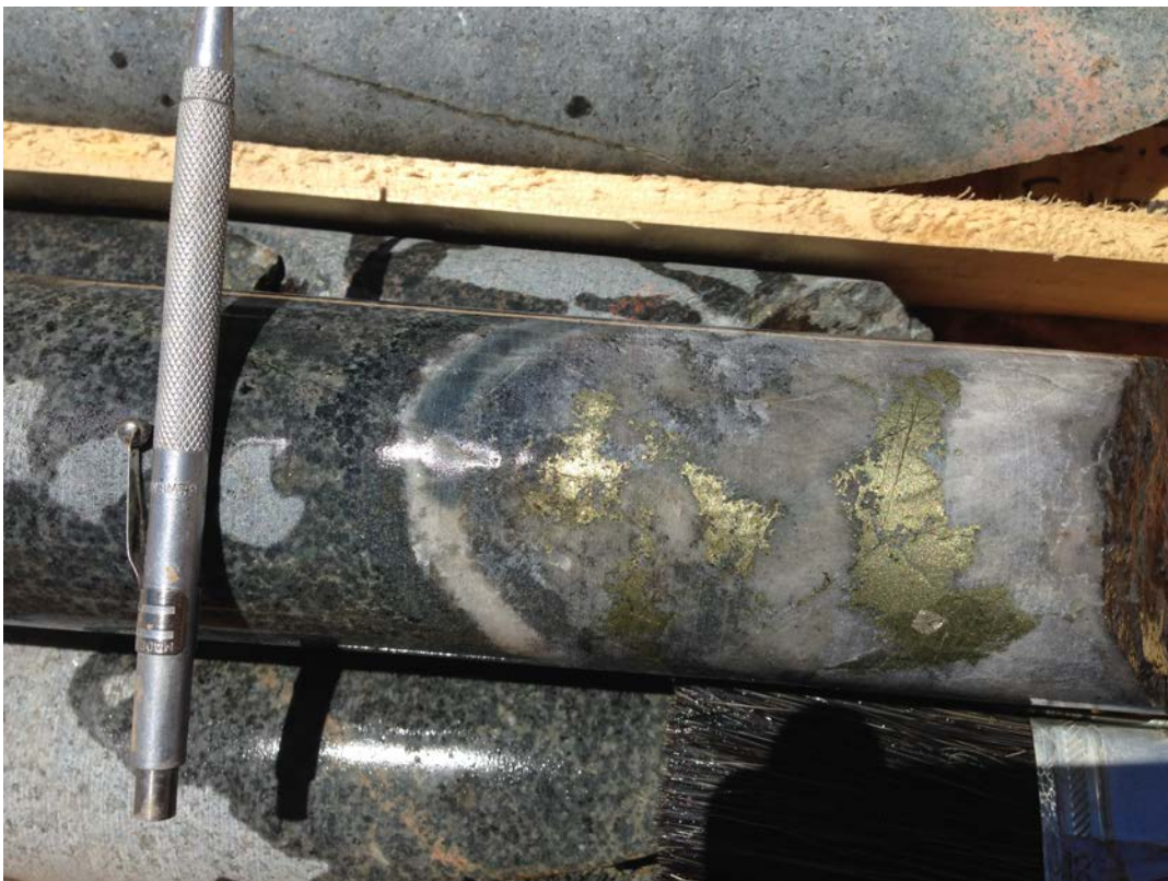
Figure 5 - Top – RCPDH00002 – 130.80- 137.50m, massive and brecciated chalcopyrite/pyrite plus quartz/calcite mineralisation outlined in yellow within strongly potassic feldspar altered diorite with up to 10% sulphide. Field of view approximately 1m.
