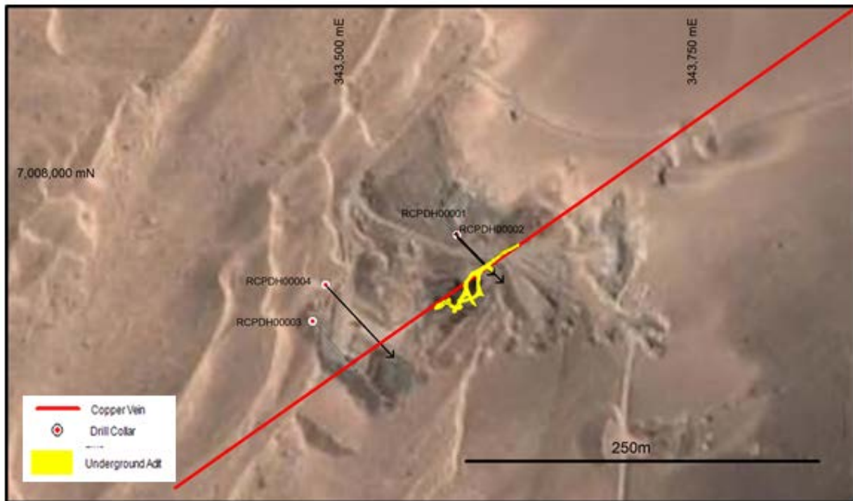
Figure 3 – Drill hole location plan over Descubridora Mine. Yellow outline depicts location of underground areas and red line depicts interpreted surface expression of the Descubridora vein.
