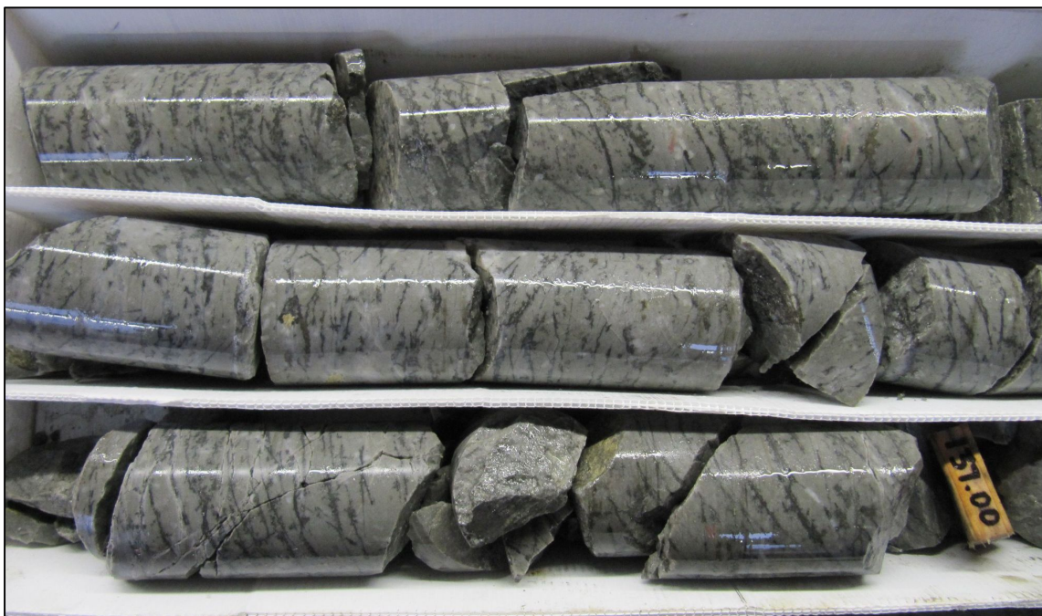
Figure 5: Drill core of moderate to high grade gold mineralisation showing fine sulphide veinlets in strongly silicified porphyry host from drill hole SCDDH088. Drill core shown averaged ~4.1g/t gold
