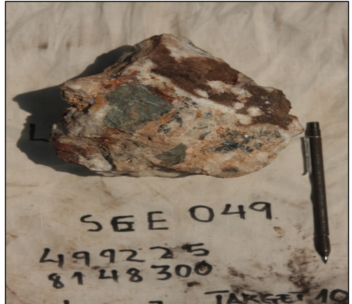
Figures 5 and 6: Hand sample of the vein collected from the Fred-Lead North Prospect. Similar to the southern outcrop, to the north the quartz vein hosts coarse galena and clasts of dolerite. Similar strike and host lithology relationships indicate the two outcrops occur along strike of the same vein.
