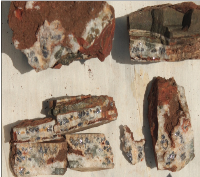
Figures 5 and 6: Hand sample of the vein collected from the Fred-Lead North Prospect. Similar to the southern outcrop, to the north the quartz vein hosts coarse galena and clasts of dolerite. Similar strike and host lithology relationships indicate the two outcrops occur along strike of the same vein.
