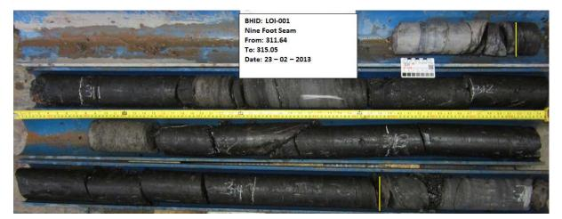
Figure 4 LOI 001 - Nine Foot Coal Seam Core 1
