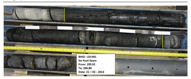
Figure 3 LOI-001 - Six Foot Coal Seam Core<sup>1</sup>
