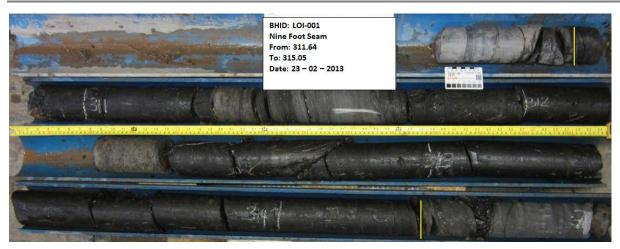
Figure 3: LOI-001 - Nine Foot Coal Seam Core<sup>1</sup>
