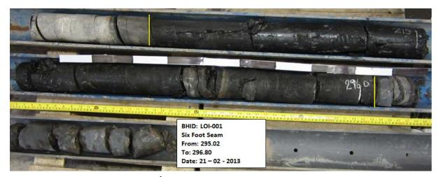
Figure 2: LOI-001 - Six Foot Coal Seam Core<sup>1</sup>
