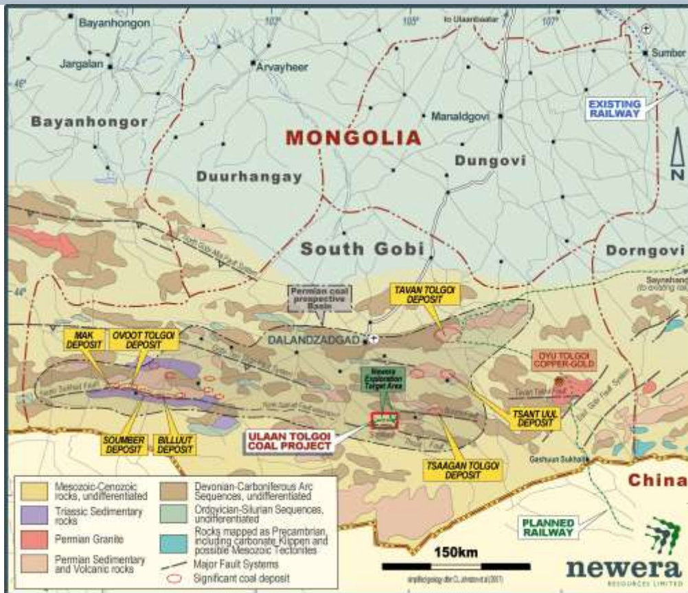
Figure 4: Ulaan Tolgoi licence area within South Gobi regional geology map – showing interpreted boundary of the Permian coal prospective South Gobi Basin – the Nariin Sukhait and Sondoult thrust faults indicated. Relevant major coal projects indicated.
